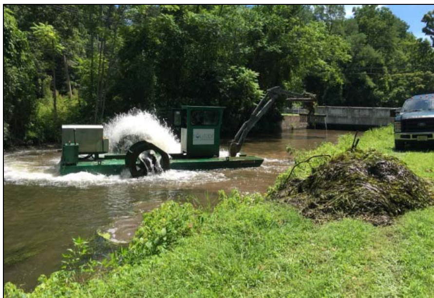
Figure 9: Hydro-raking submersed aquatic plants in the D&R Canal (2016)
