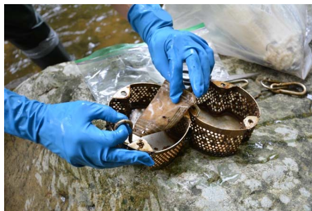
Passive cyanotoxin (SPATT) sampler, July 2021
