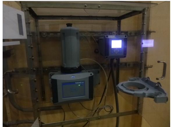
Instrumentation to determine water clarity replaced in 2017
