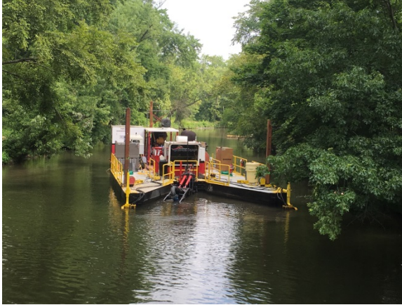
Photo shows one of three dredges currently in operation in July 2018. Note the boom extending into water in front of dredge in photo. Note three vertical square “spuds” keep equipment in place while dredging. Square plates at base of “spuds” prevent damage to clay liner at bottom of Canal. On-board computer and GPS maintain location and depth of boom and cutter head to prevent damage to the clay liner.
